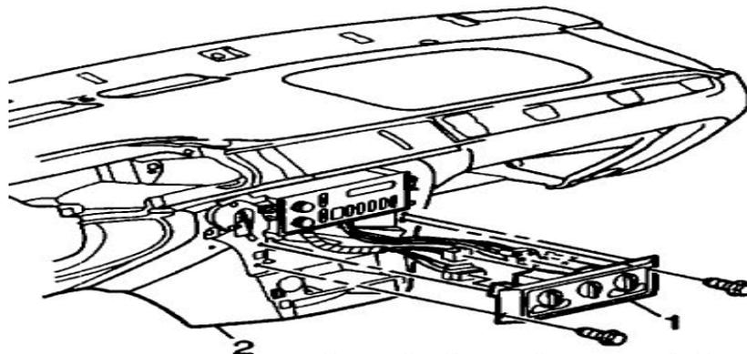
Figure 2. (1) Heater and A/C Control Assembly
